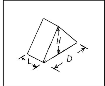
Additional pile length is the triangular portion between the cone that forms the ends of a pile that is longer than the pile diameter.
