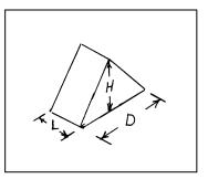
Additional pile length is the triangular portion between the cone that forms the ends of a pile that is longer than the pile diameter.
