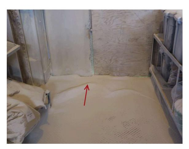
Ingredient accumulation on floor is a slip hazard
