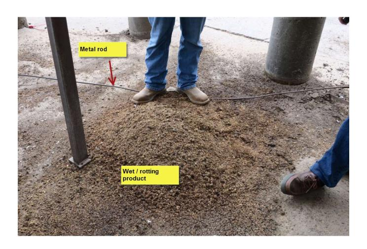
Can trip on metal bar or slip on wet/rotting grain
